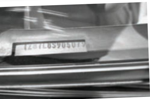
**ABOVE:** Distinguished by the "9" in the eighth digit of the VIN, this 1978 Pace Car proves to be legit. Regular production 1978 Corvettes ran from 400001 through 440274 or 40,274 Corvettes. Pace Car production added an additional 6,502 units and numbered 900001 through 906502. (Photo: Bob Stevens Archives)
