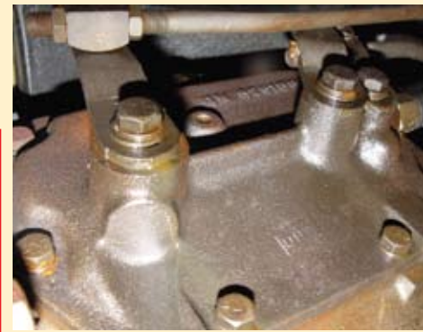
Figure 5. Muncie side cover shows three shift shafts
