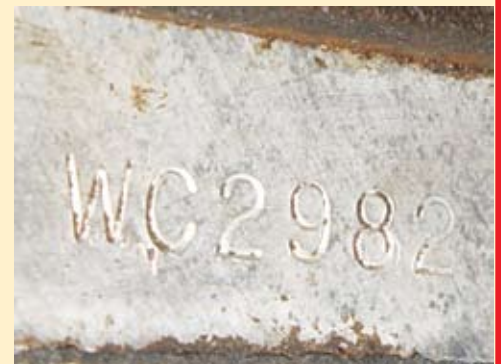
Figure 9. Borg Warner date code WC2982, assembled at the Warner plant March 29, 1978, second shift.
