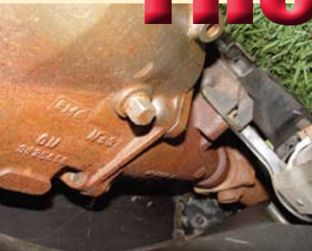
Figure 1. 1978-79 Muncie cast-iron maincase and extension housing
