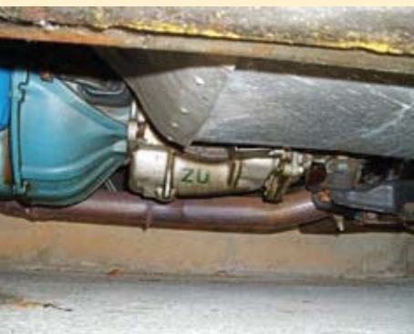
Figure 3. B/W M20 broadcast code ZU stamped on the lower half driver side of the transmission's maincase.
