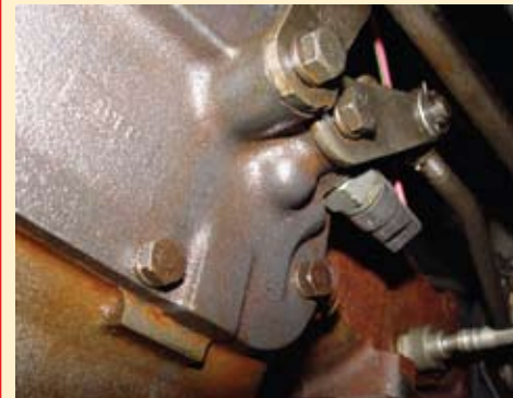
Figure 6. Muncie side cover shows location of reverse shift shaft and assembly date code pad.
