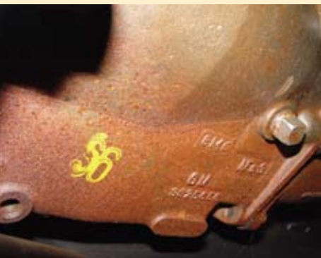
Figure 2. Muncie M20 broadcast code S6 stamped on upper front passenger side of the transmission's maincase. Photo is rotated 180° to show it upright.
