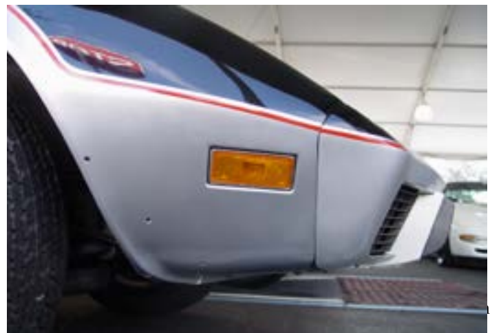
Figure 1: 1978 Pace Car as delivered to dealer without front air deflector installed.
