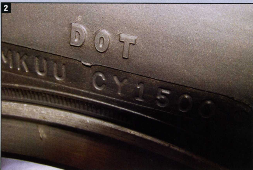
A typical 1980 P255/60R15 date code shows that tire assembly still used a single gang (actually called stencil plate) to mold the TIN into the tire. The DOT label is printed on the topside of the TIN. This tire was manufactured the 50th week of 1980.
