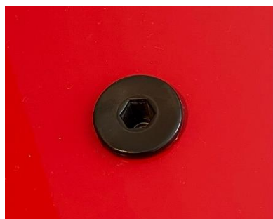
1980-82 Factory-installed deck grommet & well-nut
