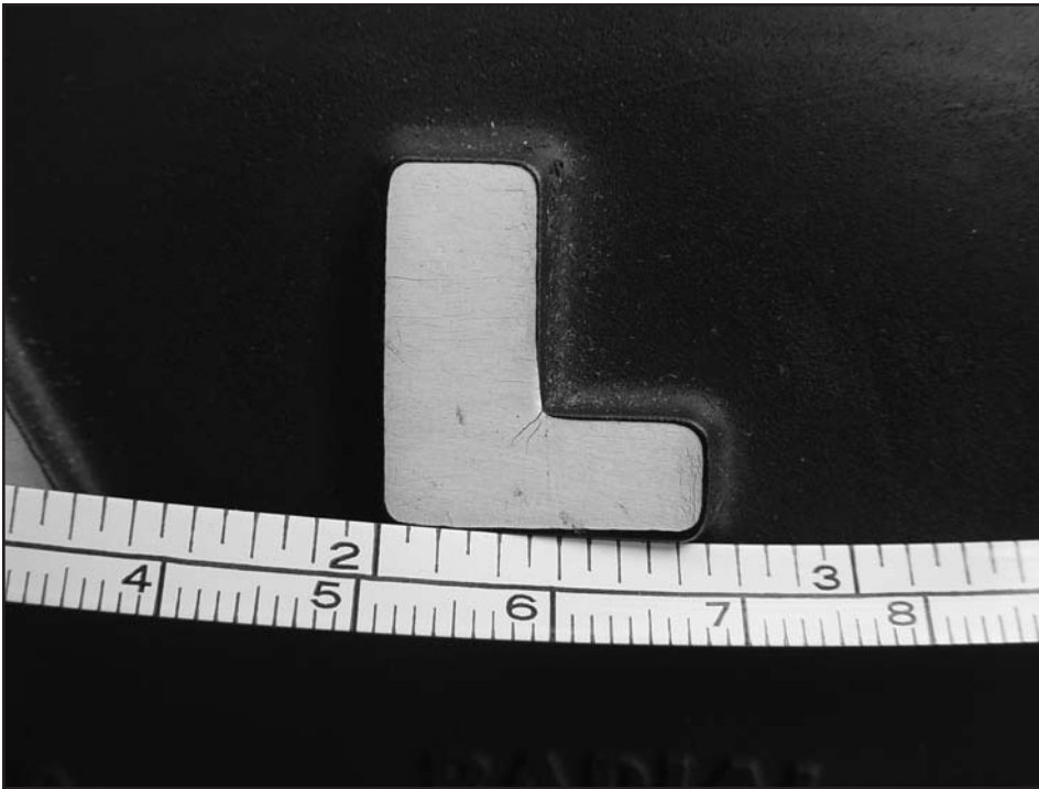
The photo at left shows a Polysteel tire with 1 st design solid white letter configuration. The "L" letter width measures 11/16"
