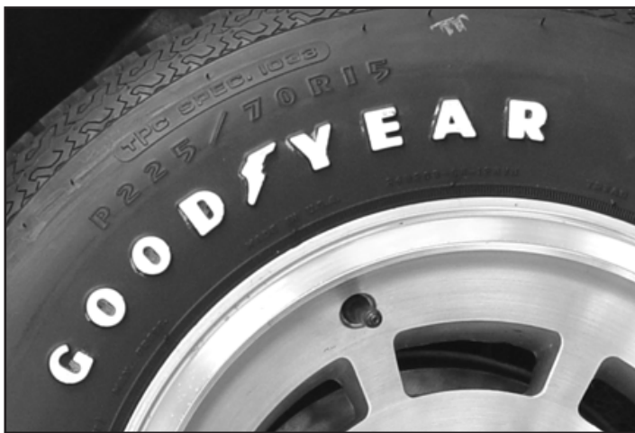
1978 Polysteel RPO QGR P225/70R15 with TPC 1033. This label is on a 1978 Corvette tire for RPO QBS (P225/70R15).
