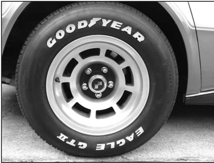
Goodyear Eagle P225/70R15 series SERVICE replacement. Note letter design, size and configuration approximates that of an original GT Radial but with bold white raised letters. Date code 1302 or 13th week of 2002.
